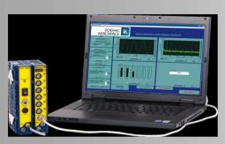
Single module system with direct link to the PC via USB 2.0
